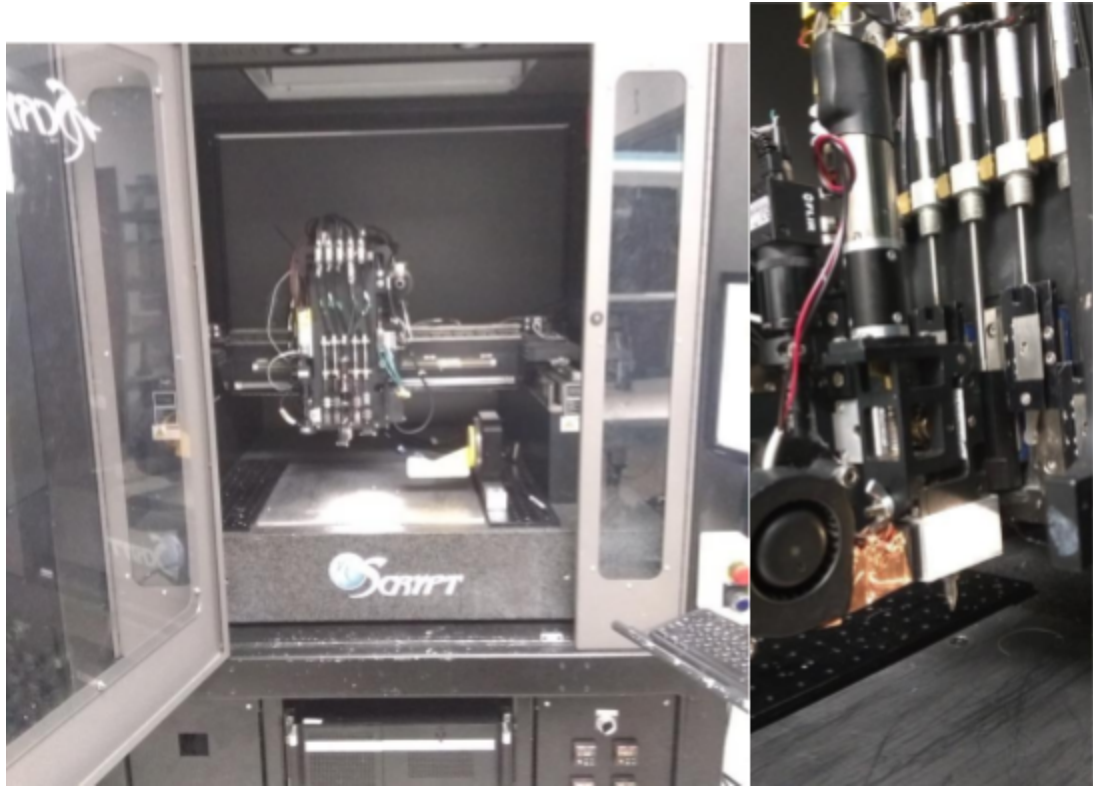
Figure 4.3.2.1: One of nScript's 3Dn Systems (left) and nFD plastic extrusion gizmo (right)
